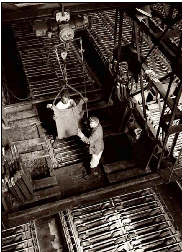
Nickel electrolysis, changing of anodes, Falconbridge Nickel Refinery (Kristiansand), 1960. Unknown photographer.
