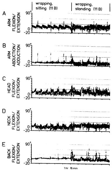
Figure 7. Postural angles from an 1 hr 16 min. recording at the 11B system, the subject first adapting a sitting, then a standing posture. Each point in the recording indicates mean angle in 0.5 second intervals.
