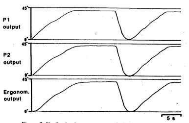
Figure 7: Similar in vitro test setup as in figure 6 for very slow movements for testing of transducer hysteresis because of internal rotational friction. Note the good correlation between the outputs. These are angular movements frequently seen at the back.
