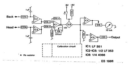
Figure 3: Electric diagram for continuous calculation of the neck angle from the head and back angles. The calibration cirquit is identical to the one shown in figure 2.
