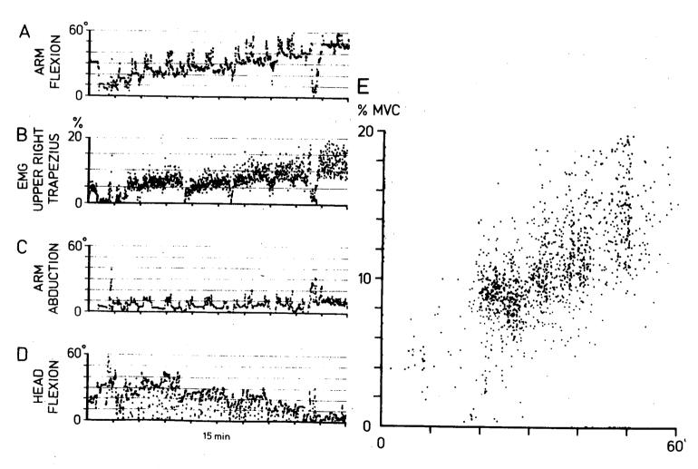
Figure 9. Arm flexion (A), EMG from upper right trapezius (B), arm abduction (C) and head flexion (D), recorded simultaneously while working at progressively higher rows at the original 8B system. Each point in the recording indicates mean angle or full-wave rectified and integrated
