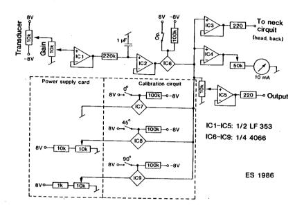
Figure 2: Electric diagram of the "Ergonometer" for head, arm and back angles. An electric calibration cirquit is shown within the interrupted lines. The RC-cirquit between IC1 and IC2 sets the time constant to about 0.2 s.
