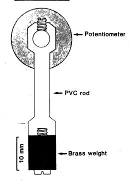
Figure 1: Schematic illustration of the potentiometer pendulum transducer. A standard Spectrol Model 157 potentiometer with a pendulum attached to the axis is used. In later versions ball bearings are applied to reduce the rotational friction.
