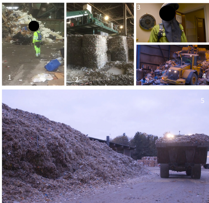
FIG 4 Picture gallery from the waste treatment plants. (1) Volunteer worker at the reception and inspection with bag pack containing sampling devices. (2) Pressed waste materials for stockage. (3) Worker with personal dust-collecting devices in the breathing zone. (4) Operating machine. (5) Bulk of waste materials for energy production.
